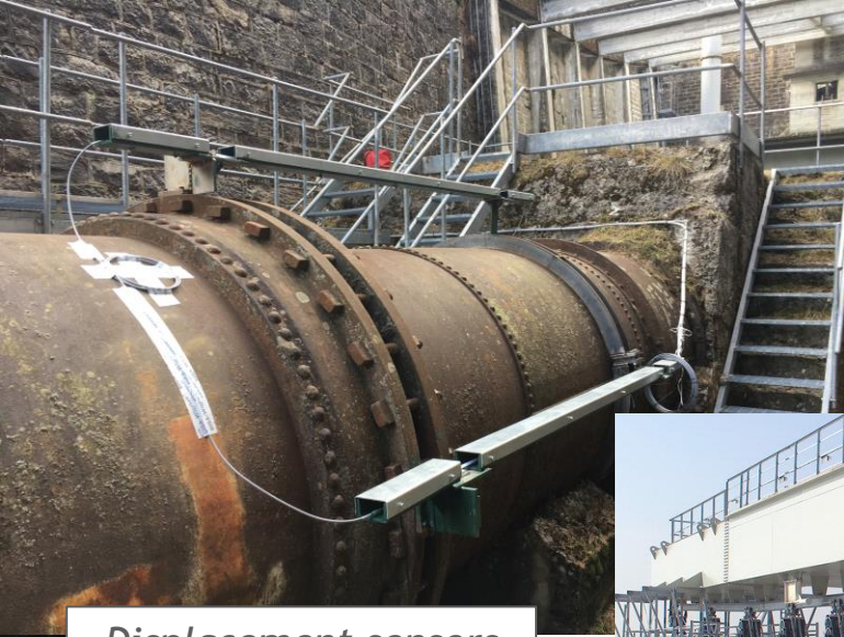
Displacement sensors along a water pipe on a landslide
