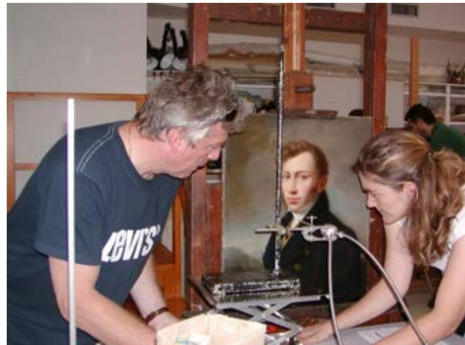
**Ten portable instruments**, XRF, FTIR, UV-VIS, Raman, etc. (7 UNIPG, 2 CNR, 1 OPD) for in-situ not invasive diagnostic on Cultural Heritage
