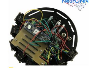
NE OSCILLATORY NEURAL NETWORKS ON FPGA FOR ROBOT OBSTACLE AVOIDANCE APPLICATION Consumer Electronics - IoT/Smart Connected Objects
