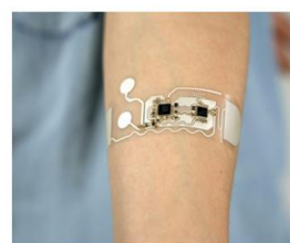
FOPE ESS ELASTIC WEARABLE ECG SKIN PATCH IoT/Smart Connected Objects - Medical/Pharmaceutical/Life Science
